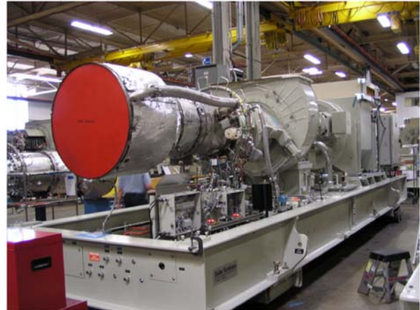
One of four 4.6MW Solar Centaur Gas Turbines for Windimurra nearing completion at the Solar Facility in Florida
